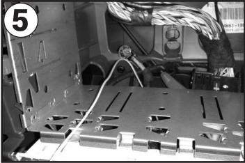
Push the metal clips on the inside of the metal cage inwards to secure the cage in the cavity
