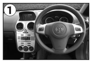
Vauxhall/Opel OEM dashboard. Ensure that the ignition is switched off before starting the installation. We also recommend that the battery is disconnected to prevent short circuits.
