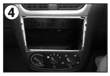
Push the metal cage into the dashboard cavity left by the factory radio
