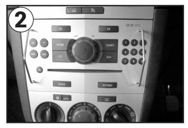
Remove the factory radio using two pairs of release keys. Push the keys into the four holes surrounding the unit to disengage the locking mechanism and remove the radio.
