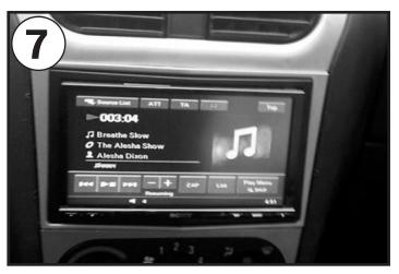
Place the aftermarket radio into the dashboard until it clips into the metal cage. Ensure that all relevant wiring is reconnected to the new radio.
