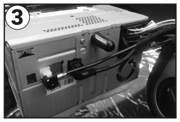
Unplug and remove the radio, taking care to remove all wiring.
